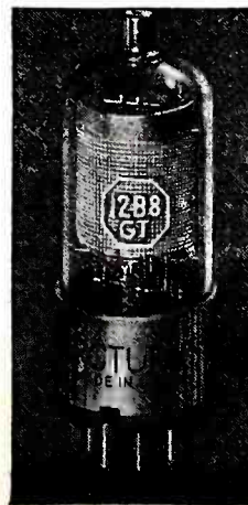
Controlled-heat crystal tube for x-mitters.
